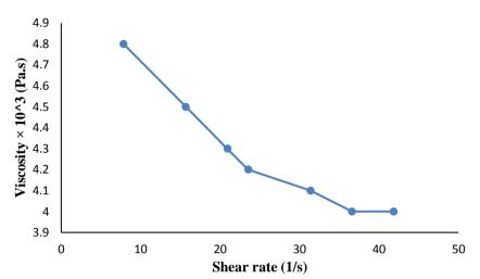
Fig.7. Viscosity values in terms of shear rate of the nano-fluid at a temperature of 50 °C.
