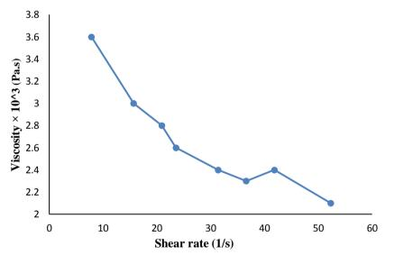
Fig.8. Viscosity values in terms of shear rate of the nano-fluid at a temperature of 65 °C.
