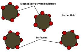
Fig.2. Magnetic nano-particles with surfactant
