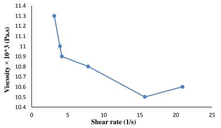
Fig.6. Viscosity values in terms of shear rate of the nano-fluid at a temperature of 35 °C.
