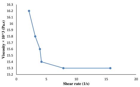
Fig.5. Viscosity values in terms of shear rate of the nano-fluid at a temperature of 20 °C.
