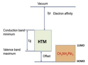
Fig 3. Schematic view of valence band offset at junction of HTM layer and perovskite.
