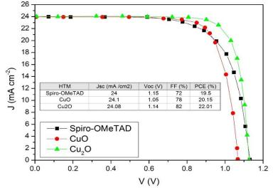
Fig 5. J-V characteristic curve and output parameters table related to simulation of the effect of applying organic and inorganic HTM layers on perovskite solar cell performance.
