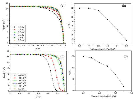
**Fig 4**. Changes in (a) current-voltage characteristic for positive offset potential values, (b) cell efficiency in terms of positive offset potential, (c) current-voltage characteristic for negative offset potential values, and (d) cell efficiency in negative offset potential.
