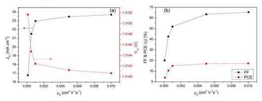
**Fig 2**. Simulated PSC performance in terms of cavity hole mobility: (a) short-circuit current and open-circuit voltage changes, and (b) FF and efficiency coefficients.
