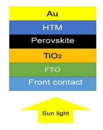
Fig 1. Simulated Perovskite Solar Cell Structure.
