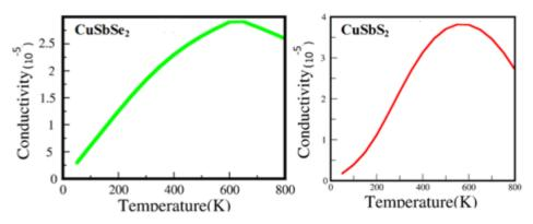
**Fig.8.** The curve of electrical conductivity in terms of temperature for CuSbSe<sub>2</sub> and CuSbS<sub>2</sub> compounds
