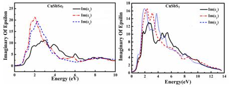
Fig.3. the imaginary part of the dielectric function in X, Y, Z directions
