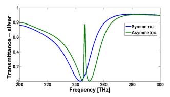
Fig. 4. Transmittance versus frequency curve of the structure in symmetrical state (blue line) and in asymmetrical state (green line),  $L_2=L_1=230$  nm,  $d_2=d_1=60$  nm.
