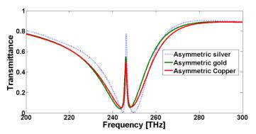
Fig. 6. The curve of Transmittance versus Frequency for Asymmetric proposed nanostructure with different metals: Silver (blue dashed lines), Gold (green line) and Copper (red line).
