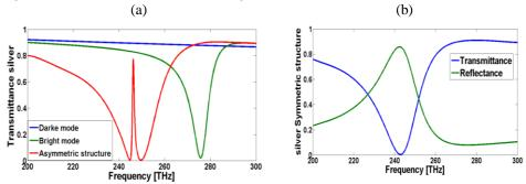
Fig. 2. a) Transmission and reflection diagrams of Silver structure, b) Transmittance versus frequency curve of Silver structure for dark mode related to  $L_1$  strip (blue line), bright mode related to  $L_2$  and  $L_3$  strips (green line) and the case of symmetry breakdown (red line).  $L_1$  and  $L_5$  equal to 225 nm,  $d_1$ =45 nm and  $d_2$ =55 nm.
