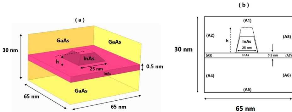
**Fig.1.** 3D schematic of our truncated pyramidal-shaped QD with wetting layer without graphene (a) with its distinct boundaries (b).
