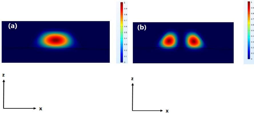
**Fig.3.** The probability density of (a) ground state (S-state) and (b) the first excited state (P-state) of a truncated pyramidal-shaped QD with the height of 7 nm and base length of 25 nm in T=0 K.
