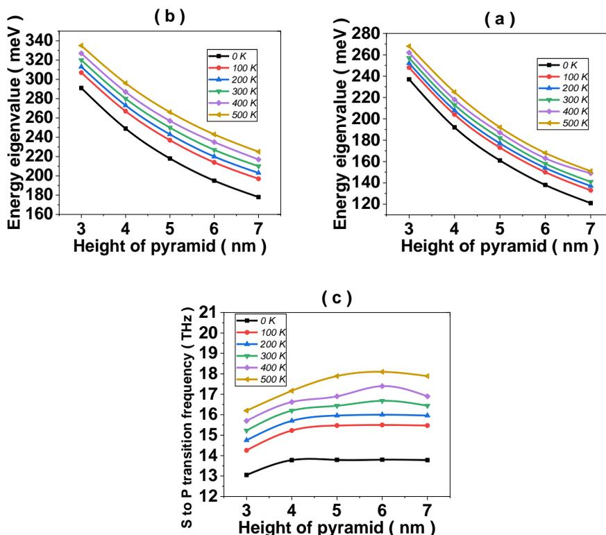
**Fig.4** (a) Energy eigenvalues of S- and P-state and (b) S-to-P transition frequency as a function of temperature and height for a QD with the constant base of 25 nm.
