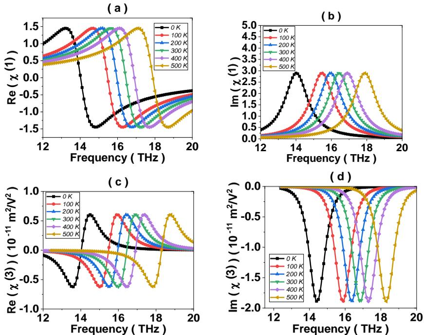
**Fig.5.** Linear susceptibility (a, b) and nonlinear susceptibility (c, d) for a pyramid with a height of 5 nm and a base length of 25 nm as a function of frequency for different temperatures.
