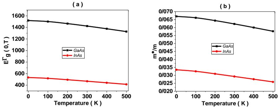
**Fig.2.** (a) The energy band gap at  $p=0$  Kbar, (b) and the ratio of effective mass to electron mass as a function of temperature.
